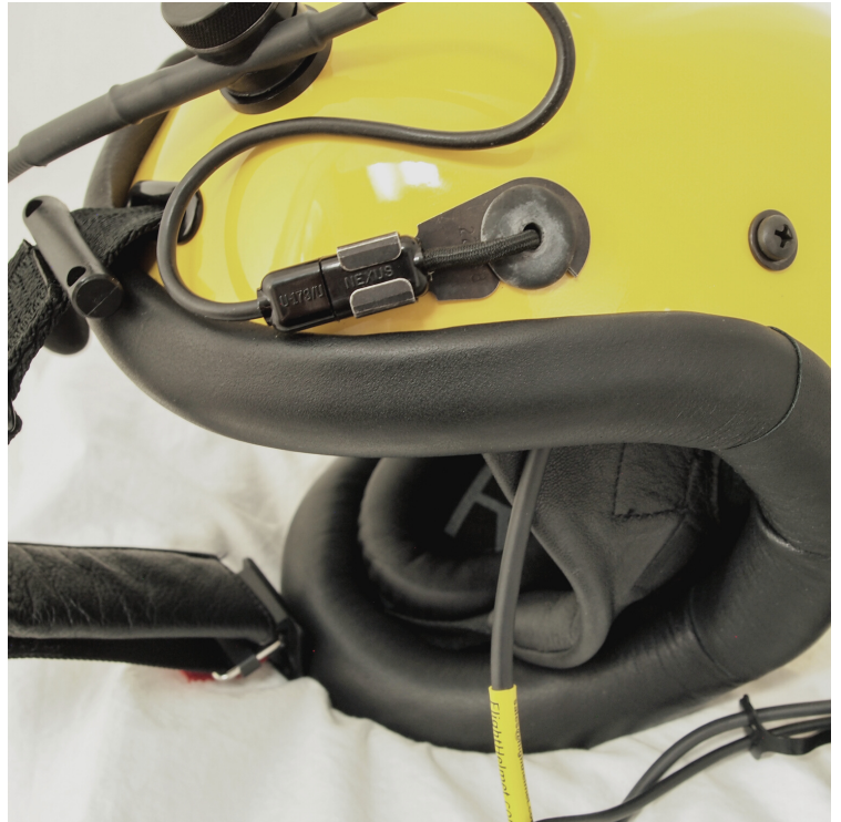
Interior of Helmet showing edge roll, ear seals, and nape strap.
